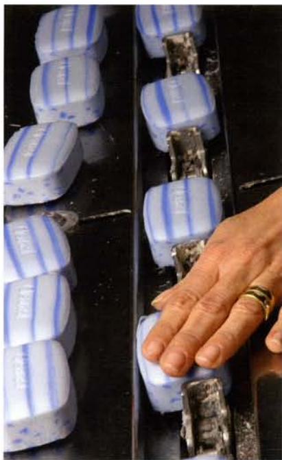
After milling, extrusion and pressing, the soap bars are conveyed, packaged and distributed.
